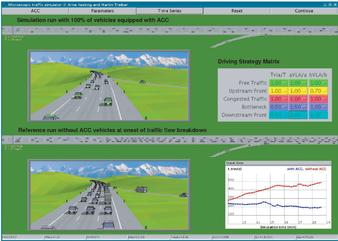
FIGURE 1 Screenshot of traffic simulator showing on-ramp scenario. Two simulation runs are displayed. In upper simulation, 100% vehicles are equipped with ACC-based traffic assistance system. Vehicle color indicates locally detected traffic state. Reference case without ACC equipment (gray vehicle) displayed in lower simulation run shows congested traffic at bottleneck. In both simulations, same time-dependent upstream boundary conditions have been used; see Figure 2.
