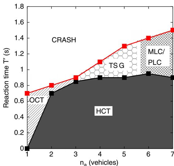
Fig. 2. Phase diagram of congested traffic states in the phase space spanned by the number  $n_a$  of anticipated vehicles and the reaction time  $T'$  in the open system with a bottleneck as described in the text. The dynamic phases homogeneous congested traffic (HCT), oscillatory congested traffic (OCT), triggered stop-and-go (TSG), and moving and pinned localized clusters (MLC/PLC) are discussed in the main text.
