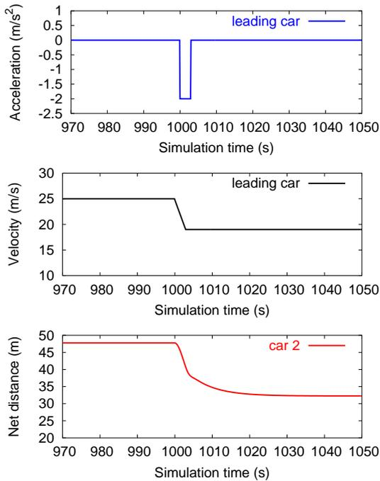
Fig. 1. Acceleration and velocity time series for the externally controlled first vehicle of the vehicle platoon. The lead vehicle decelerates at  $t = 1000$ s with  $-2$  m/s<sup>2</sup> inducing a perturbation to the platoon of vehicles. The distance of the second car is in equilibrium before the braking maneuver and adjusts to the new equilibrium distance after a while. This braking maneuver serves as perturbation in all simulations.
