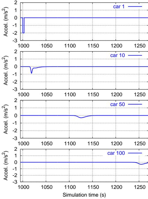
Fig. 4. Time series of the acceleration for selected platoon vehicles. The reaction time is  $T' = 0.9$ s, and the IDM parameter for the maximum acceleration is set to  $a = 1$  m/s<sup>2</sup>. The vehicles use temporal anticipation but no spatial anticipation ( $n_a = 1$ ). The first vehicle induces a perturbation due to the braking maneuver at  $t = 1000$ s. The initial perturbation do not increase while propagating through the platoon of vehicles. The system is string stable.
