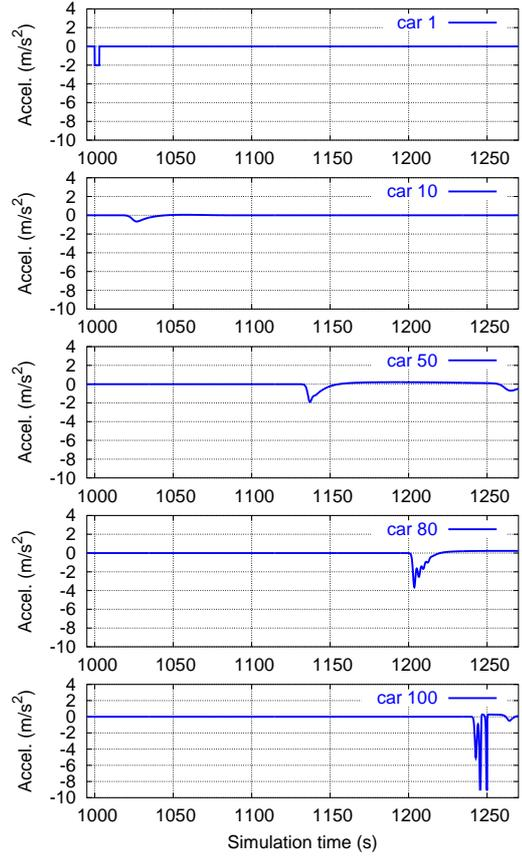
Fig. 5. Time series of the acceleration for the same scenario as in Fig. 4, but the IDM parameter for the maximum acceleration is reduced to  $a = 0.3$  m/s<sup>2</sup>. The initial perturbation caused by the braking maneuver of the first vehicle is firstly reduced (car 10), but finally increases while propagating upstream resulting in a stop-and-go wave for the car 100. More stop-and-go waves are triggered as shown in Fig. 6.
