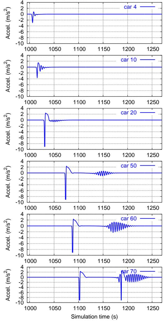
Fig. 7. Time series of the acceleration for the same scenario as in Fig. 4, but the IDM parameter for the maximum acceleration is increased to  $a = 2.5 \text{ m/s}^2$ . Again, the first vehicle induces a perturbation due to the braking maneuver at  $t = 1000 \text{ s}$  (not shown here). The increased acceleration parameter  $a$  in combination with the delayed reaction causes higher frequencies with periods about 4 s that finally trigger stop-and-go-waves of a much higher period (about 50 s).
