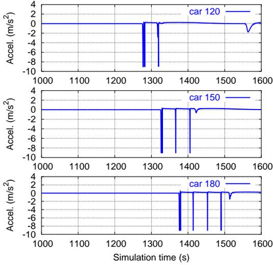
Fig. 6. Patterns of stop-and-go waves. The simulation is identical to that of Fig. 5, but vehicles further upstream are shown on a different time scale. The period of the stop-and-go waves is about 40 s.
